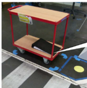
The red cart in every Hancho Team shows the problems on the shop floor.
